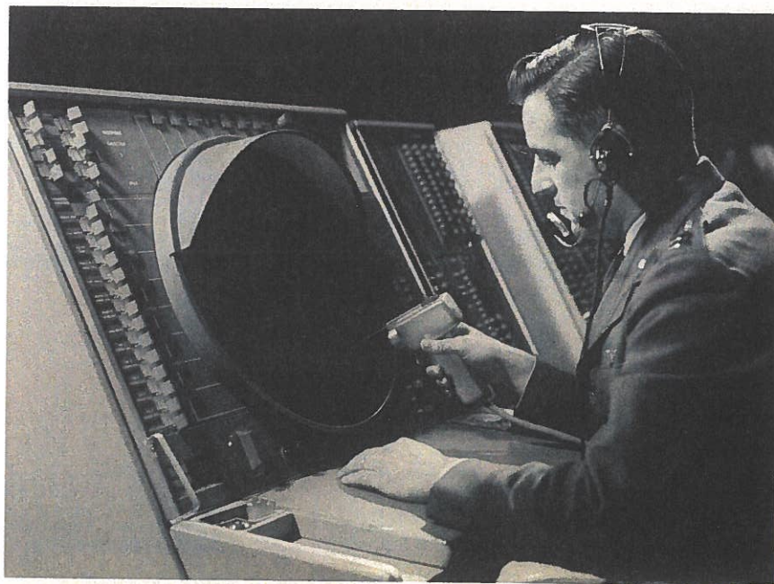
Figure 9.4 Operators of SAGE used light guns to pinpoint aircraft tracks. When a blip appears on the scope, the light beam causes the computer to assign a track number and to relay speed, direction and altitude information to various consoles. Publicity photograph of a SAGE console operator with 'gun' pointed at the screen. 1959 ca.
